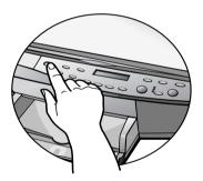
When your HP PSC 500 is on, text appears in the front-panel display. If you do not see a message, check the power cord connections from the back of the unit to the power-supply adapter and from the power-supply adapter to the power outlet.
